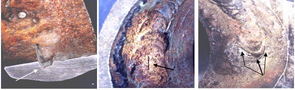
Fig.1 Lack of fusion in weld of pipe (Ø38, thick-3mm)
