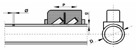
Fig.5 Calibration block examination of pipe weld (thickness-g, diameter of reference hole ø =1mm, D-pipe diameter, P- direction of probe movement for DAC
