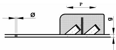
Fig.4 Calibration block of flat element (thickness-g ,diameter of reference hole ø =1mm, P- direction of probe movement for DAC
