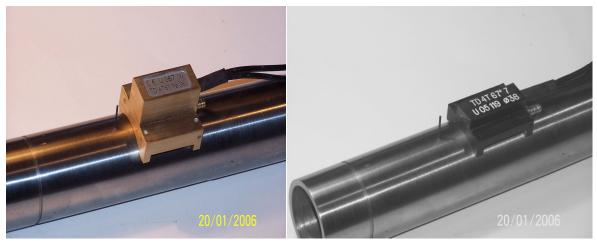
Fig.9 The profiled tandem probe in brass casing
