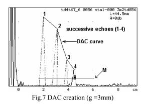
In modern flaw detectors the DAC curves are stored with appropriate FD set-ups according to procedures pointed in IBUS-TD instruction. In older FD the DAC curve can be drawn on transparent foil placed on the FD screen. It can be used many times but it requires writing extra data for identification. The working parameters of FD during DAC creation should be kept the same during examinations - otherwise it can lead to unacceptable errors.
