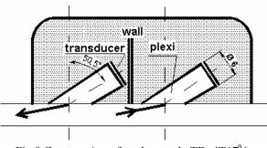
Fig.8 Construction of tandem probeTDx4T67<sup>0</sup>6
