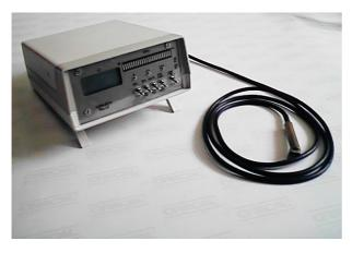
The meter measures both strength and spatial gradient of static magnetic field. The operator can adjust the amplification level of field strength measurements. The measurement of spatial gradient of the magnetic field strength near the steel surface allows quick detection of crack. Apart from being displayed numerically, the signal of spatial gradient is visualized on a light bar indicator and translated into a frequency modulated sound. The voltage signals are redirected to output
