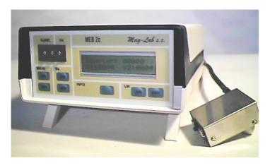
The meter measures three quantities: the Barkhausen effect (BE) signal voltage effective level, the number of BE pulses and control voltage amplitude of signal. The amplification of BE voltage analyser and BE pulses threshold counter level differential adjustable. The measurement of effective voltage allows detection of local change of BE properties. Three output
