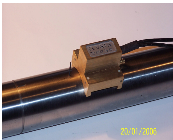
Figure 4. Tandem probe with CE notation, U067 (Ultra No.), DM (big, brazen casing), TD 4T67 7, Ø38, with cosy handle, reference hole has stick inside.
