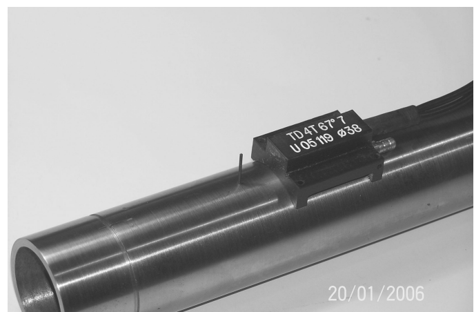
Figure 5. Tandem probe with CE notation, U067 (Ultra No.), PM (small, plastic casing), TD 4T67 7, Ø38, height about 10 mm, reference hole has stick inside.
